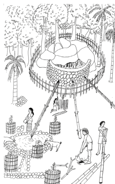
Gravity fed water supply and irrigation
